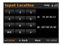
Note, the format used to enter the location is set by the button in the lower right corner of the screen. In this example, we show coordinates using DMS format.
