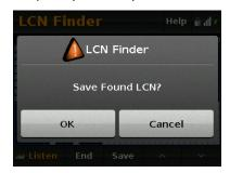
Note that because this process uses statistical correlation, it can result in *false finds*, especially on a busy system. It is a good idea to run this process several times and compare results before saving an LCN map for a system. Best results are achieved when the system is not extremely busy.
