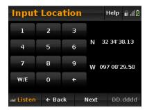
Note, the format used to enter the location is set by the button in the lower right corner of the screen. In this example, we show coordinates using DMS format.
