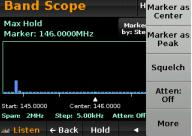
Marker as Center – rescales the frequency range to set the position of the marker as the center frequency.
