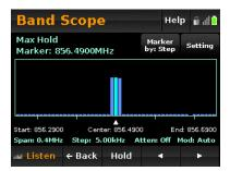
Finally, we've determined that the signal is at about 856.485 MHz. The signal is about 20 kHz wide (the bar in the middle of the signal is at a minimum level because it falls off the 5 kHz step being used).
