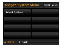
If you did not select to use the current system, enter the first part of the name of the system you want to analyze. The system must be in the systems currently selected for scanning.
