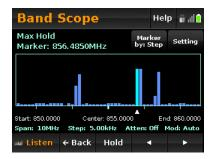
Now, set Marker as Center to center the range on the peak signal and narrow the span. In this case, the span is narrowed to 2 MHz.
