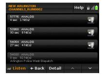
Hits for found channels include a recording of the audio during that hit. Tap the row to play back the audio.
