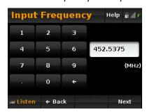
Enter the LCN for the frequency and tap Accept. If you do not know the LCN assignment, enter any LCN not used for another frequency, then later use the LCN Finder function to adjust the assignments.
