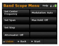
Set Center Frequency – set the frequency at the center of the frequency range you want to analyze.
