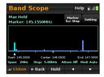
Tap the left and right arrows at the bottom of the screen to adjust the position of the marker at the bottom of the analyze window. Tap Marker by: above the display to change how the marker moves:
