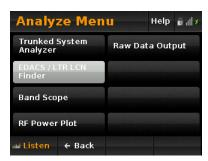
If you were last scanning an EDACS or LTR system, you have the option of using the current system, or selecting a system to analyze.
