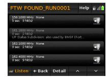
Hits for found channels include a recording of the audio during that hit. Tap the row to play back the audio.
