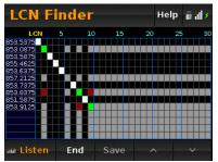
White cells are cells with high LCN to frequency activity and are likely LCN matches.
