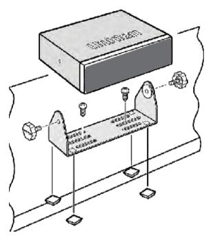
To secure the radio to a surface by means of the mounting bracket, follow the steps below:
