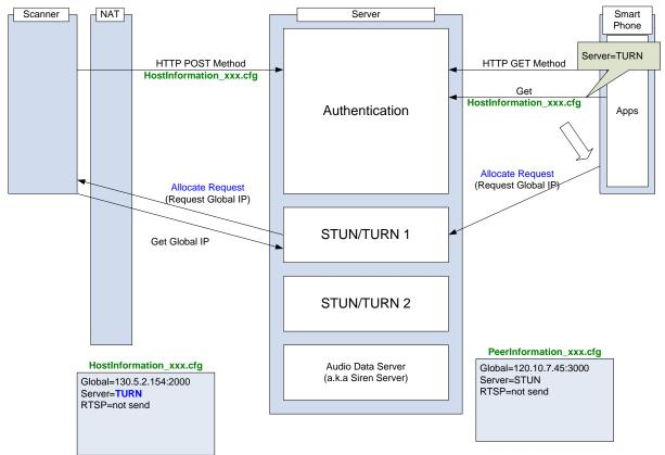
TURN Server return Global IP Address and Port Number when Scanner send Allocate Request (refer to RFC5766 / <u>http://tools.ietf.org/html/rfc5766</u>) to STUN/TURN Server. Scanner describes Global IP Address and Port Number and kind of Server:[Server=TURN], and upload HostInformation\_xxx.cfg by using HTTP POST method to Authentication Server. If Scanner is [Server=TURN] and Smartphone's App is [Server=STUN], Smartphone's App switch to TURN Server by the following method.
