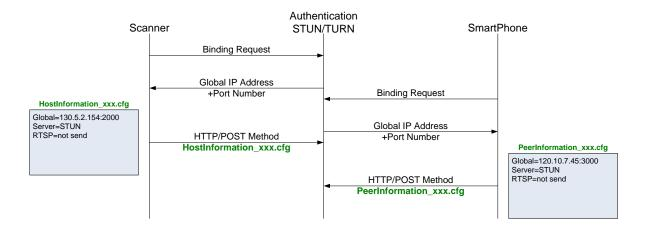
Scanner will send Binding Request to two or more of the STUN / TURN server with different address.
