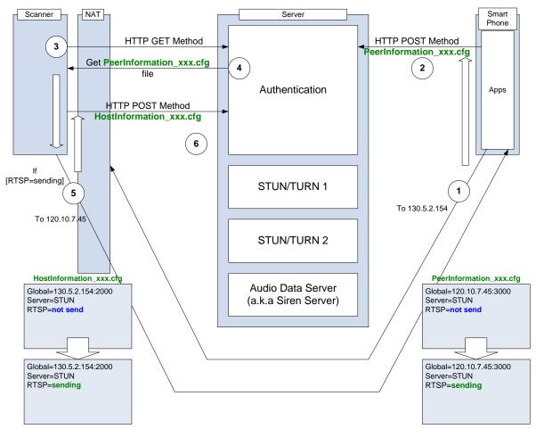
Also, if it is (Port) Restricted cone NAT, Scanner can't receive the RTSP Method from App if Scanner doesn't transmit once for Global IP Address of Smartphone's App.
