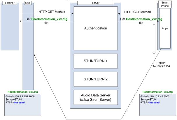
Smartphone's App start transmitting the RTSP to the Scanner's Global IP Address described in the HostInofrmation\_xxx.cfg file.
