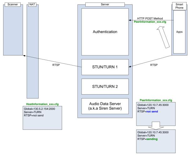
If Scanner receives OPTIONS method (RTSP data) from TURN Server, update to [RTSP=sending], and upload HostInformation\_xxx.cfg by using HTTP POST method to Authentication Server.
